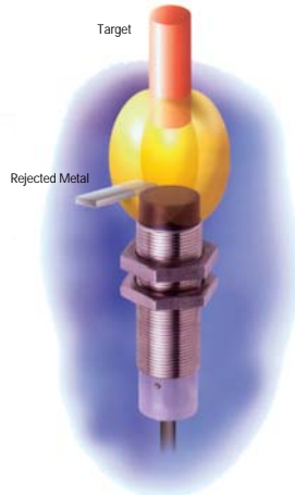
Program Background Rejection: MyProx ignores metal objects on the side, fore- and background.*
