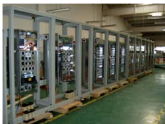
Drive and Inverter engineering and panel building
